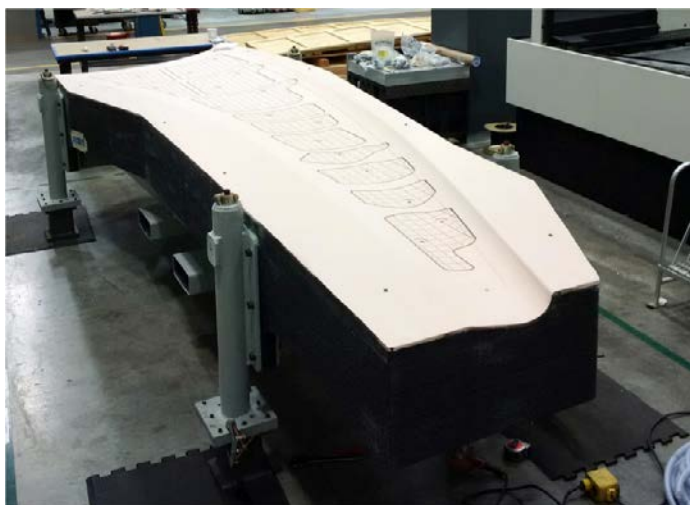
Figure 9: 3D Printed Wing trim for Boeing 777x (17.5 ft long, 5.5 ft wide and 1.5 ft tall) (Alec, 2016)
